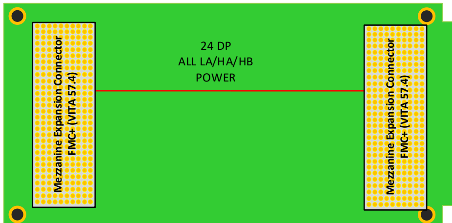
Figure 5: FMC000 Functional Block Diagram
