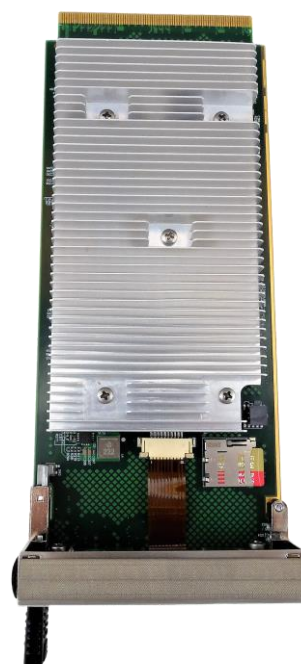
Figure 2: AMC332 with Heatsink
