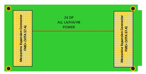
Figure 5: FMC001 Functional Block Diagram
