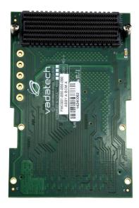
Figure 3: FMC001 Top View
