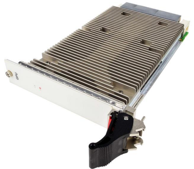
Figure 2: VPX100 with Rear I/O
