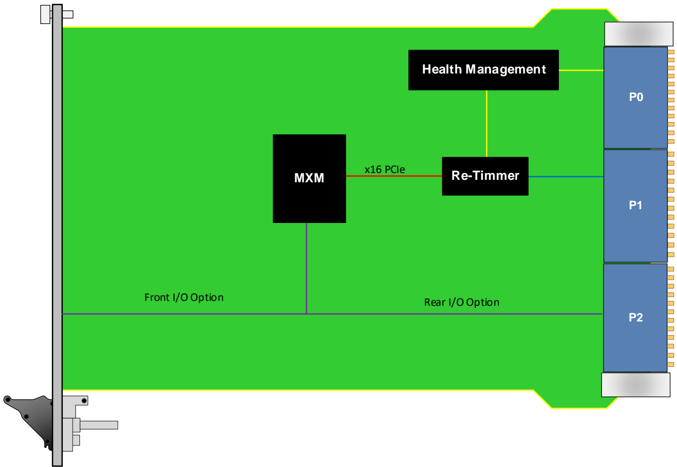
Figure 3: VPX100 Functional Block Diagram
