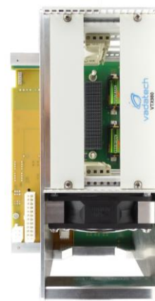
Figure 6: Chassis Layout – Rear Vertical
