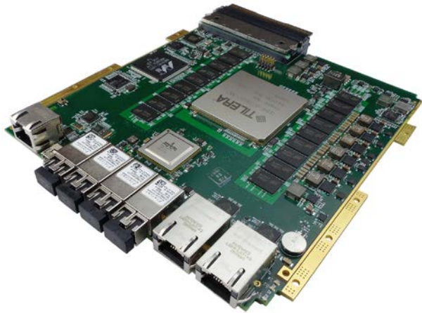
2. By using a second connector “tongue,” additional I/O and power pins are available, as in this AMC from VadaTech.
