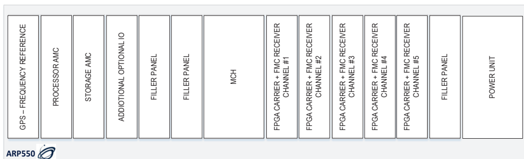
Figure 2: Architecture Block Diagram of the loaded MicroTCA Chassis Platform
