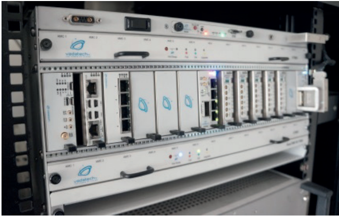
Figure 3: Loaded MicroTCA chassis platform
