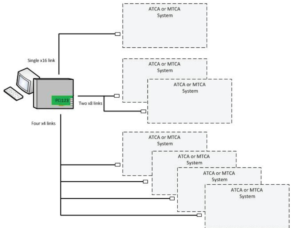
**Figure 1:** Remote PC links up to 500m using fiber
