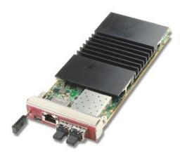
Pre-configured as a TCP Offload Engine, this AMC provides socket layer services to a Cavium OCTEON CN56xx/CN57xx Multi-Core processor, and can be loaded either by a four-lane PCIe interface or optional flash memory. This host processor enables the AMC220 to process Ethernet packets at line rate while reducing the overhead associated with new standards for packet processing on embedded CPUs.
