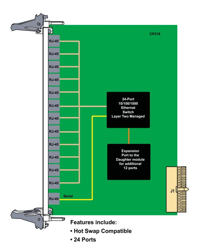
FIGURE 1. CP218 Functional Block Diagram
