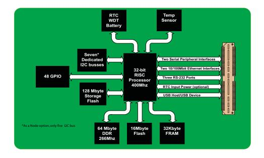
FIGURE 2. VT002 Functional Block Diagram
