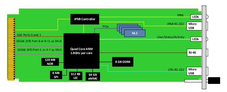
Figure 3: AMC613 Functional Block Diagram
