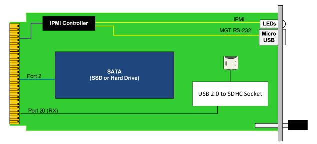
Figure 1: AMC619 Functional Block Diagram
