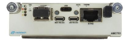
Figure 3: AMC753 Front Panel
