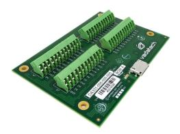
DA331 is a breakout module for the Oculink x4 cable style.
