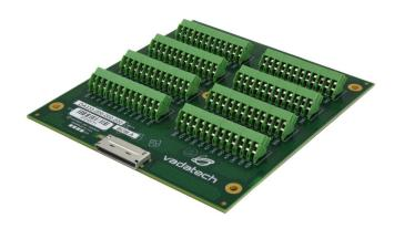
DA333 is a breakout module for the Oculink x8 cable style.
