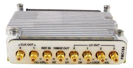
Figure 5: FMC164 Front Panel
