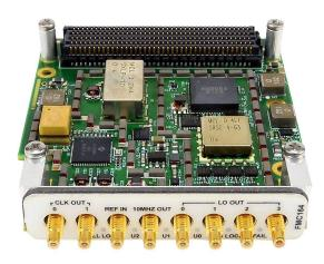
Figure 3: FMC164 without Heat Sink
