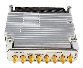
Figure 2: FMC164 with Heat Sink
