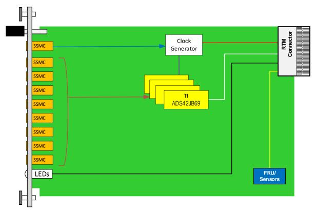
Figure 4: MRT566A Functional Block Diagram
