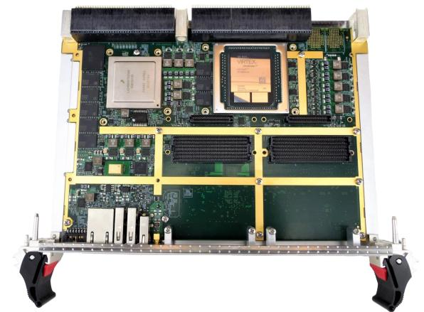
Figure 4: VPX554 Top View without Heatsink
