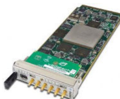
AMC526 AMC Dual ADC, Virtex-7, 12-Bit @ 2.6 GSPS
