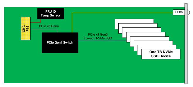
Figure 2: XMC645 Functional Block Diagram
