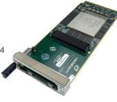
VITA 57 FMC slot, making it ideal for implementing external system interfaces at the edge of an emulation network. The KU115 is the largest of the Kintex UltraScale™ FPGAs with over 5,500 DSP slices and GTH (16.3Gb/s) transceivers.
