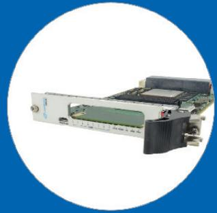
OpenVPX FPGA Carrier for VITA standard FMC+ XCZU19EG on VPX580 with double FMC+ sites (left) XCZU15EG on VPX581 with single FMC+ site (right)
