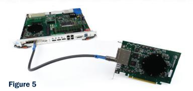
capability of massive throughput. The PCI123 can also be connected to an AdvancedTCA system. Figure 5 shows a expansion module connected to an ATCA PCIe Gen3 carrier. In the MicroTCA format there is also an option to plug to a rugged chassis directly. The VT951 is a 1U rugged chassis designed to meet MIL-STD-810G and 901D for shock and vibration. The chassis has far superior
