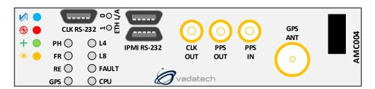
Figure 3: AMC004 Front Panel
