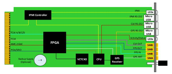
Figure 2: AMC004 Functional Block Diagram
