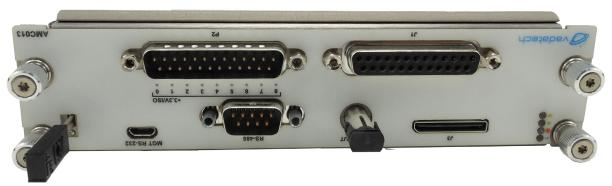
Figure 2: AMC013 Front Panel
