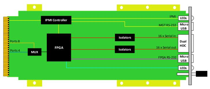
Figure 3: AMC081C Functional Block Diagram
