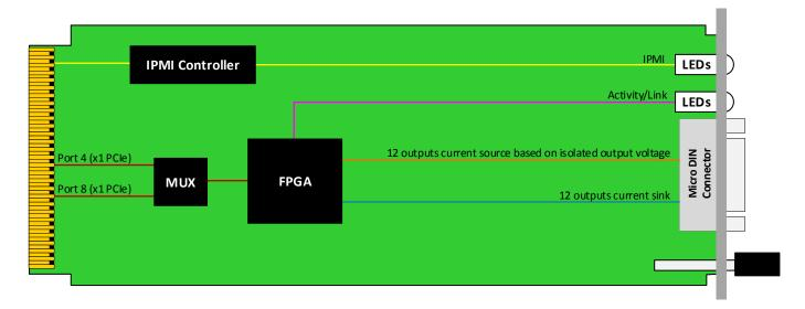
Figure 1: Block Diagram
