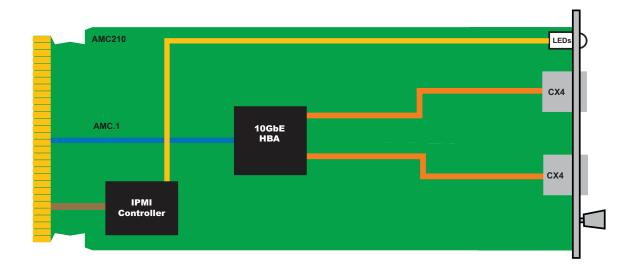
FIGURE 1. AMC210 Functional Block Diagram
