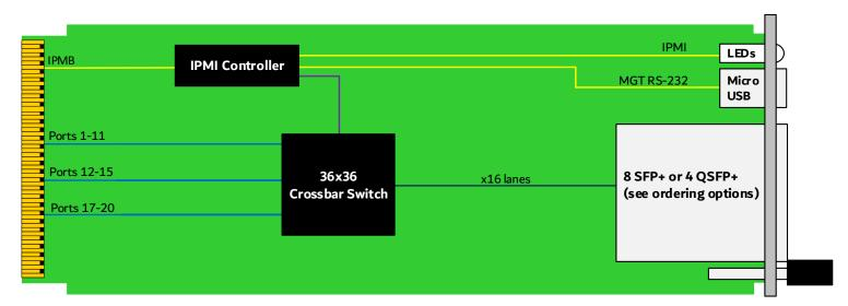
Figure 3: AMC241 Functional Block Diagram
