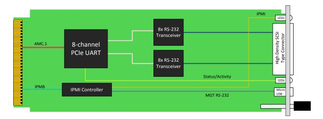
Figure 1: AMC304 Block Diagram and Front Panel
