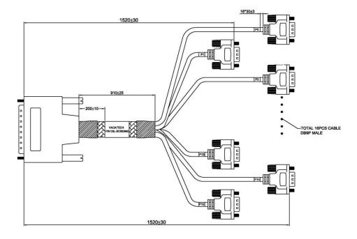
Figure 2: Diagram of Optional Adapter Cable
