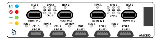
Figure 3: AMC350 Front Panel
