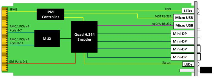
Figure 2: AMC351 Functional Block Diagram
