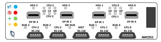
Figure 3: AMC351 Front Panel
