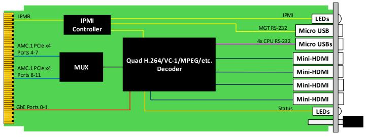
Figure 2: AMC352 Functional Block Diagram
