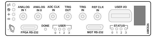
Figure 2: AMC526 Front Panel
