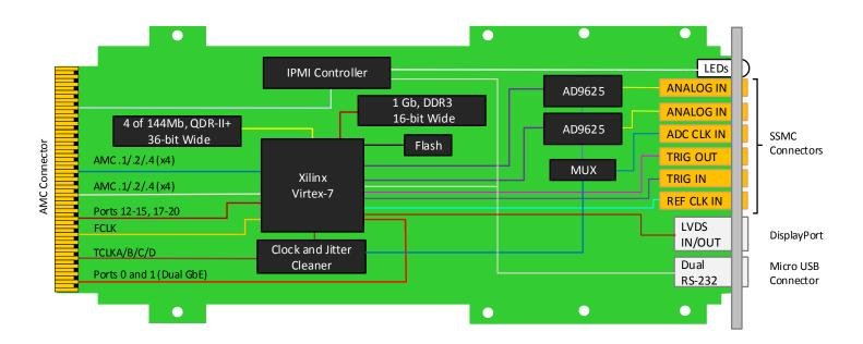
Figure 3: AMC526C Block Diagram
