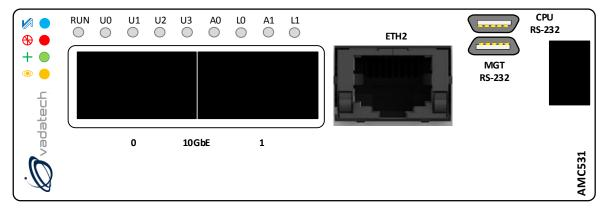
Figure 3: AMC531 Front Panel
