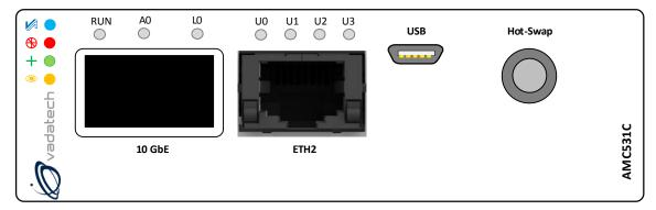
Figure 5: AMC531C Front Panel
