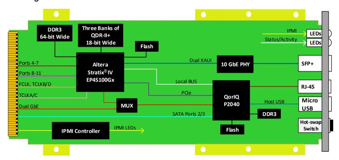
Figure 4: AMC531C Functional Block Diagram
