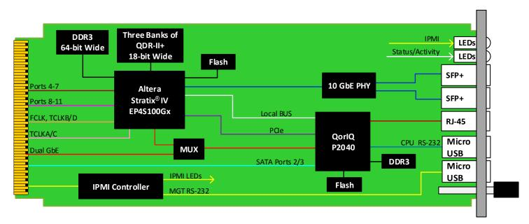
Figure 2: AMC531 Functional Block Diagram
