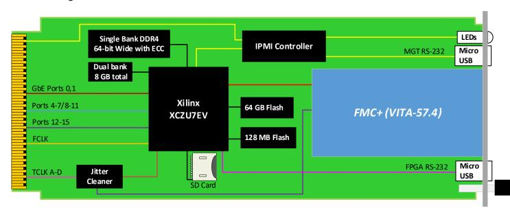
Figure 2: AMC582 Functional Block Diagram
