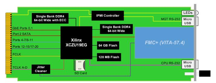
Figure 2: AMC585 Functional Block Diagram
