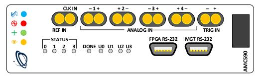
Figure 3: AMC590 Front Panel
