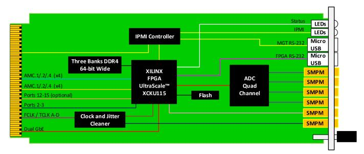
Figure 2: AMC590 Functional Block Diagram
