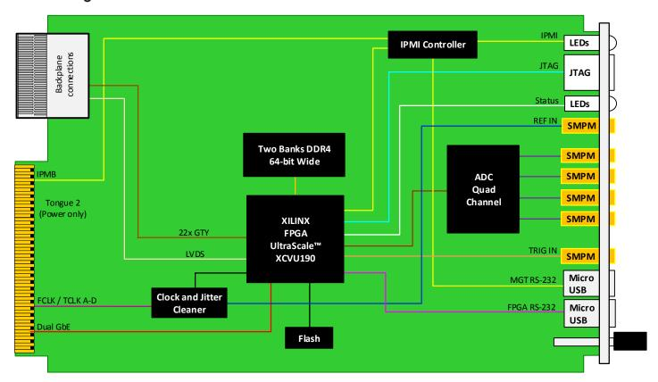
Figure 3: AMC594 Functional Block Diagram
