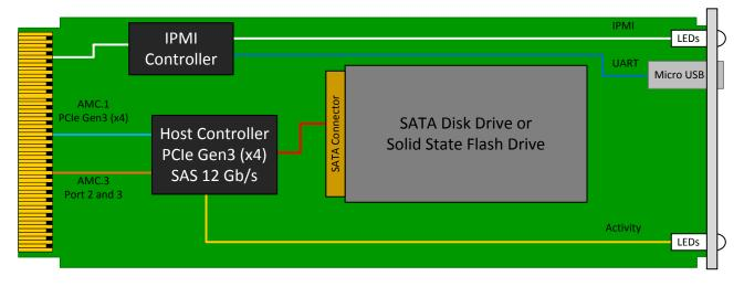
Figure 1: Block Diagram
