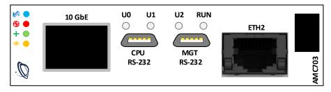
Figure 3: AMC703 Front Panel
