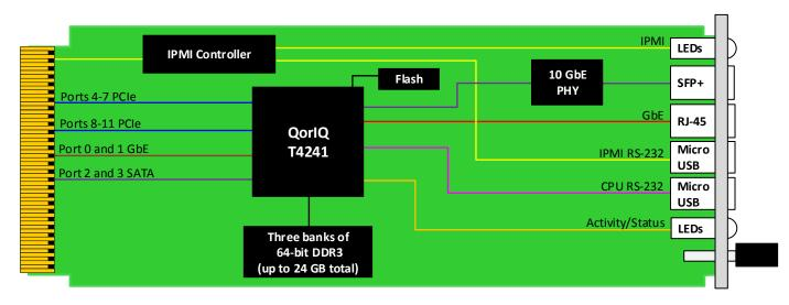
Figure 2: AMC703 Functional Block Diagram
