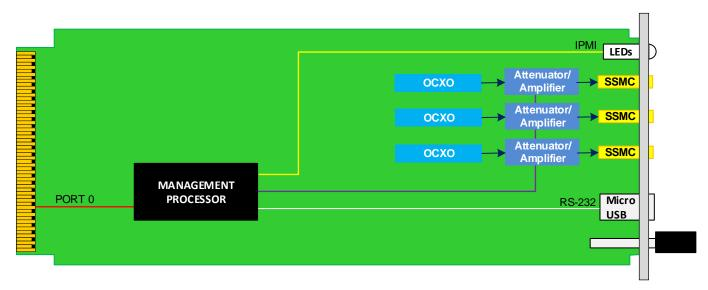
Figure 2: AMC903 Functional Block Diagram
