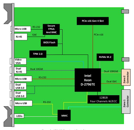
Figure 2: ATC125 Functional Block Diagram
