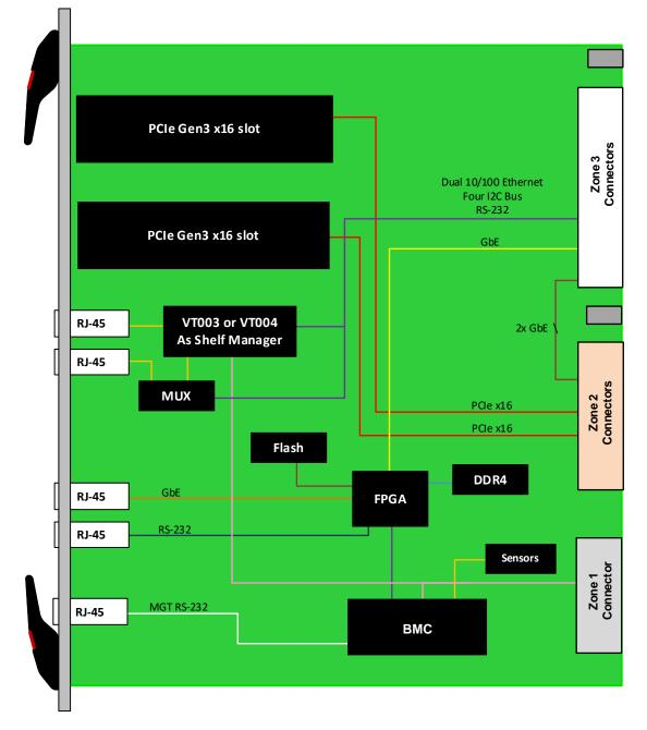
Figure 2: ATC130 Functional Block Diagram
