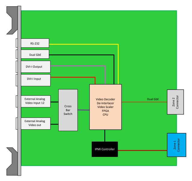
Figure 1: ATC342 Block Diagram
