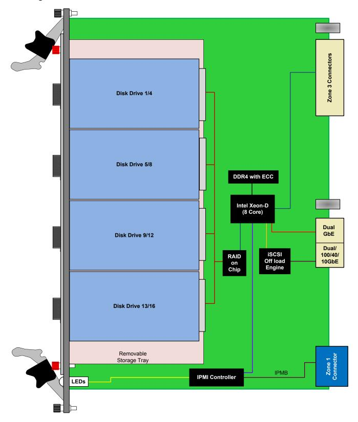
Figure 4: ATC600 Functional Block Diagram
