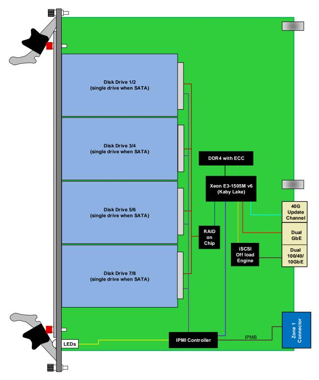
Figure 2: ATC605 Functional Block Diagram
