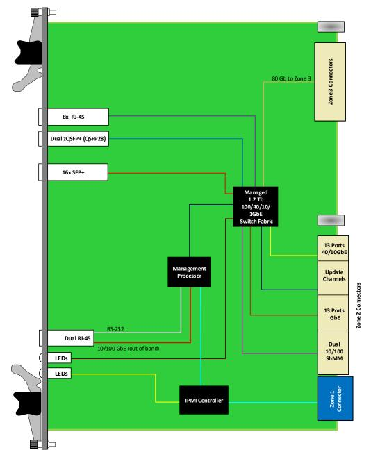
Figure 2: ATC804 Functional Block Diagram
