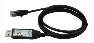
CBL002 is a 1 meter adaptor cable for connecting a PC running terminal emulation to VadaTech products that use a RJ-45 for RS-232 console I/O (which includes air-cooled MCH and OpenVPX platform management modules).
